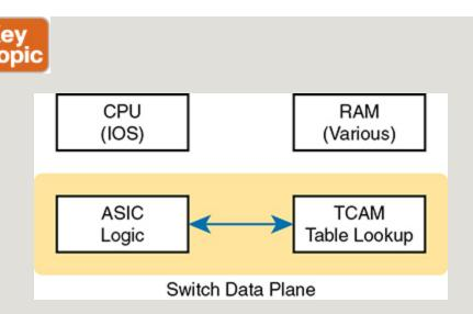
**Figure 16-4** *Key Internal Processing Points in a Typical Switch*
