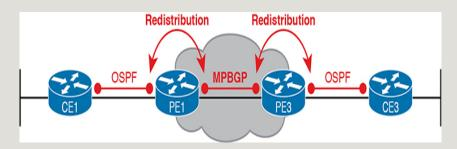
**Figure 14-15** *MPLS VPN Using Redistribution with MPBGP at PE Router*
