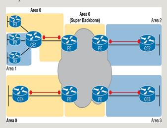
**Figure D-21** Using Area o on CE-PE Link, or for Entire Site
