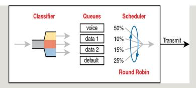
**Figure 11-16** Round Robin Not Good for Voice Delay (Latency) and Jitter
