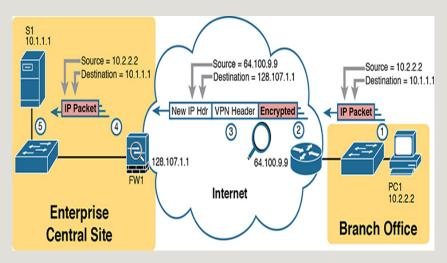
**Figure 14-20** VPN Tunnel Concepts for a Site-to-Site Intranet VPN
