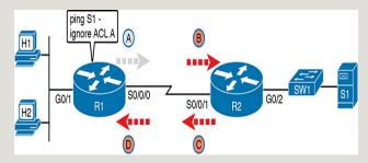
**Figure D-7** R1 Ignores Outgoing ACL for Packets Created by Its Own **ping** Command
