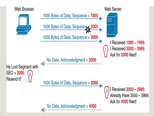
Figure 1-8 TCP Acknowledgment with Errors
