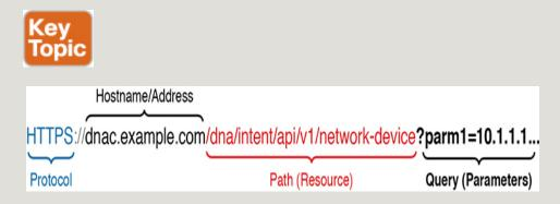
**Figure 18-8** Example Components of a URI Used in a REST API Call
