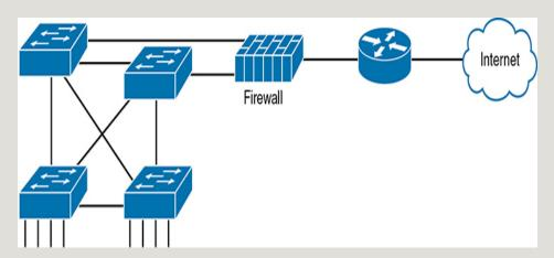
**Figure 5-5** Firewall as Positioned in the Packet Forwarding Path
