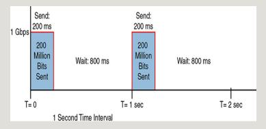
**Figure 11-21** One Second (1000 ms) Shaping Time Interval, Shaping at 20 Percent of Line Rate
