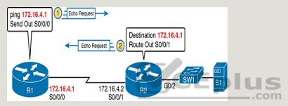
**Figure D-8** The First Steps in a Self-Ping on R1, for R1's So/o/o IP Address
