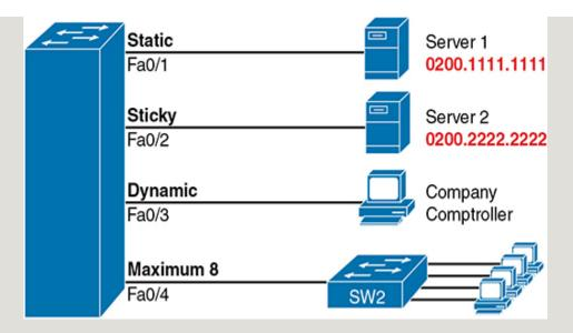
Figure 6-2 Port Security Configuration Example
