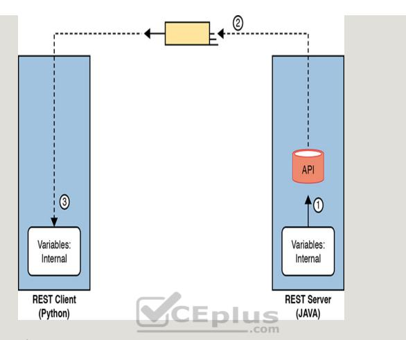
**Figure 18-10** Broken Concept: Exchanging Internal Representations of Variables
