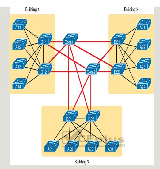
**Figure 13-5** Three-Tier Building Design (Core Design), Three Buildings
