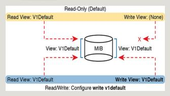
**Figure D-14** SNMPv3 Views Creating Read-Only and Read-Write Effect
