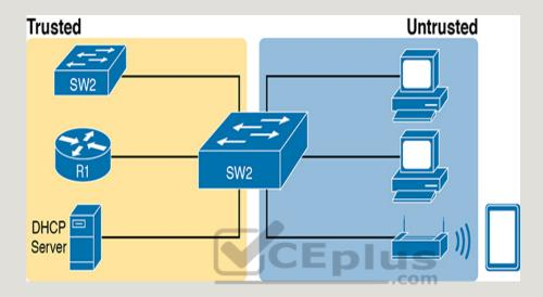
**Figure 8-1** *DHCP Snooping Basics: Client Ports Are Untrusted*
