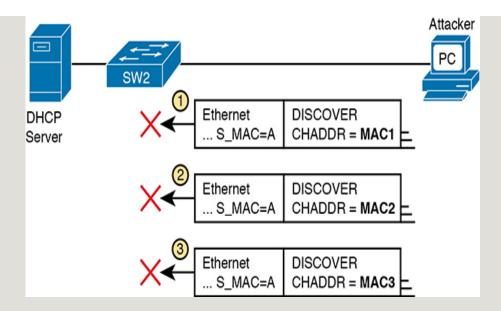
**Figure 8-5** *DHCP Snooping Checks chaddr and Ethernet Source MAC*
