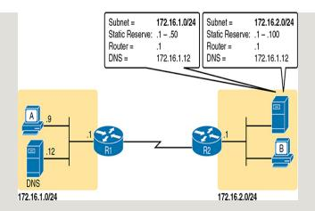
Figure 7-4 Preconfiguration on a DHCP Server
