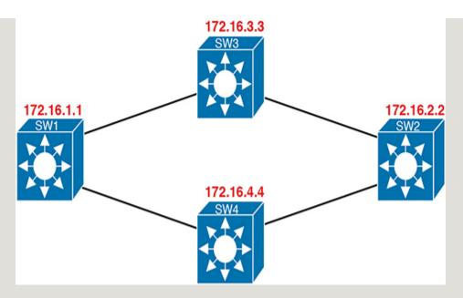
Figure 17-6 SDA Underlay Using 172.16.0.0
