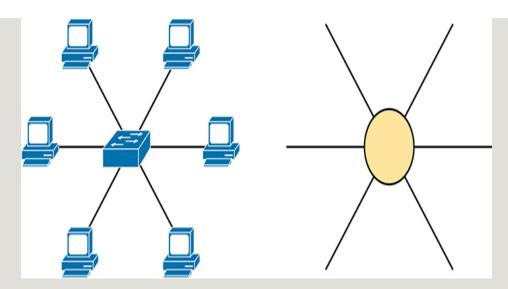
**Figure 13-2** The Star Topology Design Concept in Networking
