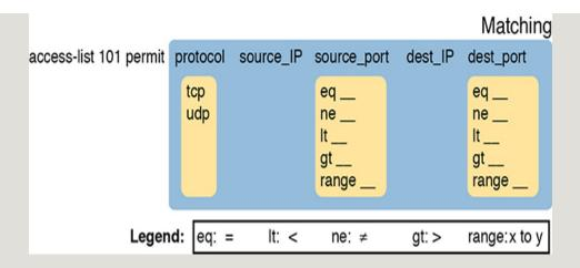
**Figure 3-5** Extended ACL Syntax with TCP and UDP Port Numbers Enabled
