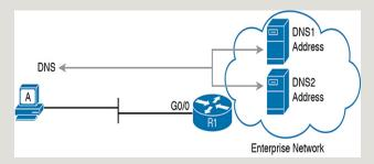
**Figure 7-6** Host A Needs to Know the IP Address of the DNS Servers
