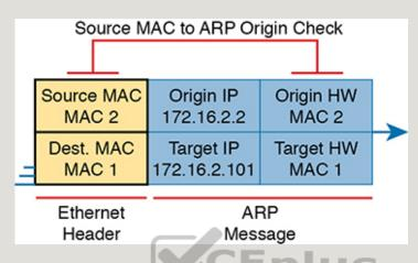
**Figure 8-14** *DAI Filtering Checks for Source MAC Addresses*
