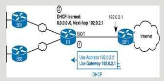
**Figure 7-5** Enterprise Router Building and Advertising Default Routes with DHCP Client
