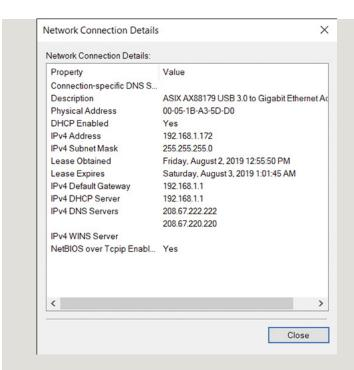
**Figure 7-9** *IP Address, Mask, and Default Router Settings on Windows*
