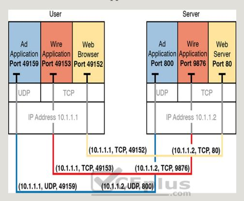
Figure 1-4 Connections Between Sockets
