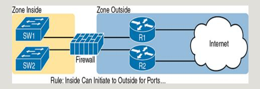
**Figure 5-7** *Using Security Zones with Firewalls*
