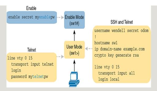
Figure 5-1 Sample Login Security Configuration
