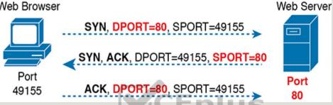
Figure 1-5 TCP Connection Establishment
