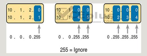
**Figure 2-6** Logic for WC Masks 0.0.0.255, 0.0.255.255, and 0.255.255.255
