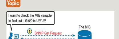
**Figure 12-9** SNMP Get Request and Get Response Message Flow
