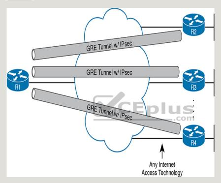
**Figure 14-22** Site-to-Site VPN Tunnels with GRE and IPsec
