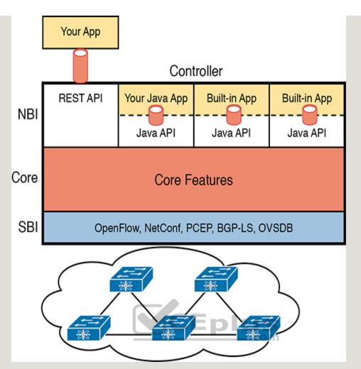
**Figure 16-8** Architecture of NBI, Controller Internals, and SBI to Network Devices
