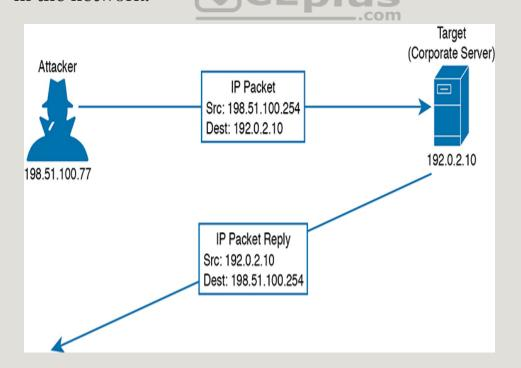
Figure 4-4 A Sample Spoofing Attack
