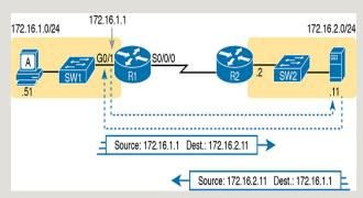
**Figure D-4** Addresses Used Between Relay Agent and Server
