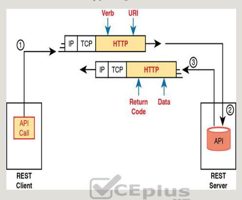
Figure 18-1 Client/Server Operation with REST
