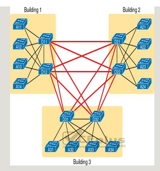
**Figure 13-4** *Two-Tier Building Design, No Core, Three Buildings*
