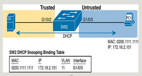
**Figure 8-6** Legitimate DHCP Client with DHCP Binding Entry Built by DHCP Snooping
