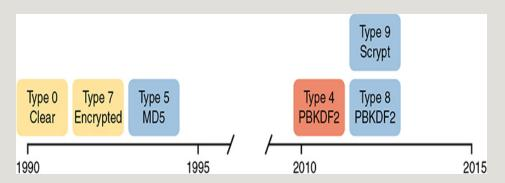
**Figure 5-4** Timeline of Encryptions/Hashes of Cisco IOS Passwords
