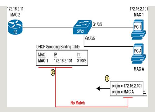
**Figure 8-13** *DAI Filtering ARP Based on DHCP Snooping Binding Table*
