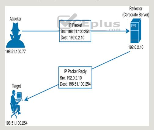
Figure 4-6 A Sample Reflection Attack
