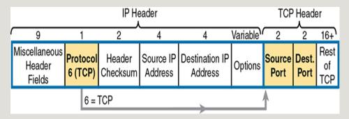
**Figure 3-4** *IP Header, Followed by a TCP Header and Port Number Fields*
