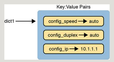
Figure 18-3 Dictionary Data Structures in Python
