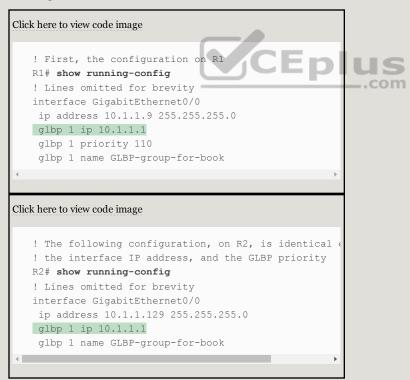
Once configured, the two routers negotiate as to which will be the AVG. As with HSRP, if both come up at the same time, R1 will win, with a priority set to 110 with the **glbp 1 priority 110** command versus R2's default priority of 100. However, if either router comes up
