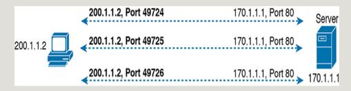
**Figure 10-7** Three TCP Connections from One PC
