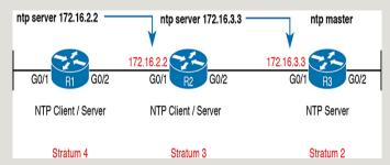
**Figure 9-5** R1 as NTP Client, R2 as Client/Server, R3 as Server
