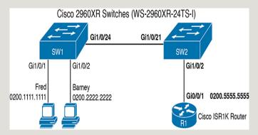
Figure 9-8 Small Network Used in CDP Examples
