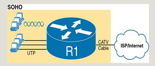
Figure 13-7 A Typical Home Wired and Wireless
