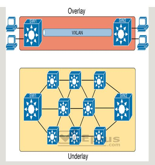
**Figure 17-2** Fabric, Underlay, and Overlay Concepts
