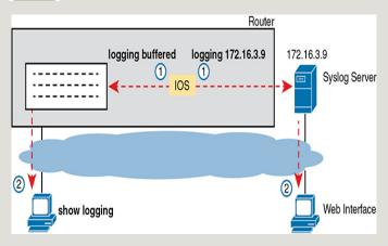
**Figure 9-2** IOS Storing Log Messages for Later View: Buffered and Syslog Server
