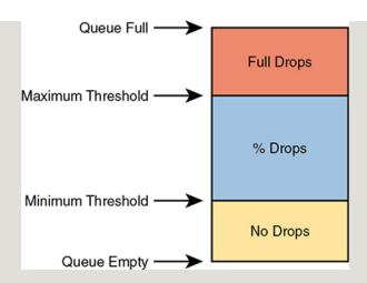
Figure 11-23 Mechanisms of Congestion Avoidance
