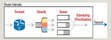
**Figure 11-3** Big Idea: Classification for Queuing in a Router
