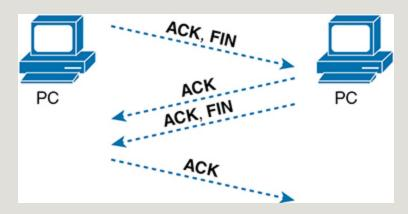
Figure 1-6 TCP Connection Termination
