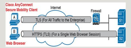
Figure 14-23 Remote Access VPN Options (TLS)
