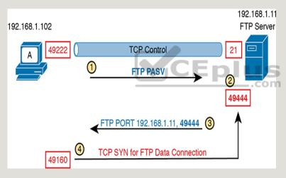
**Figure 12-19** FTP Passive Mode Process to Create the Data Connection
