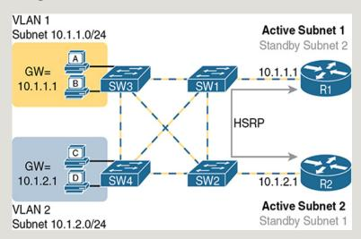
**Figure 12-7** Load Balancing with HSRP by Using Different Active Routers per Subnet
