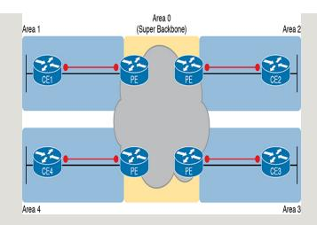
**Figure D-20** MPLS Design with (Super Backbone) Area o, Non-Backbone Area for Each Site
