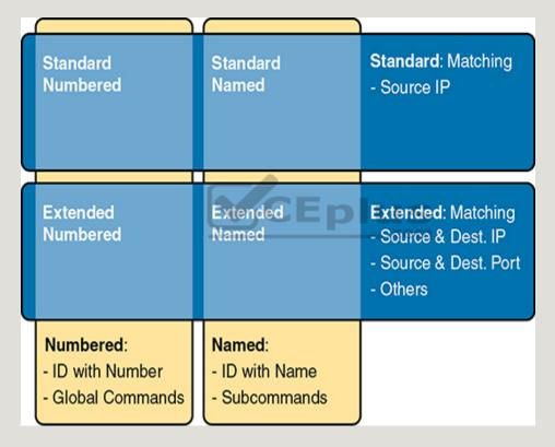
Figure 2-3 Comparisons of IP ACL Types
