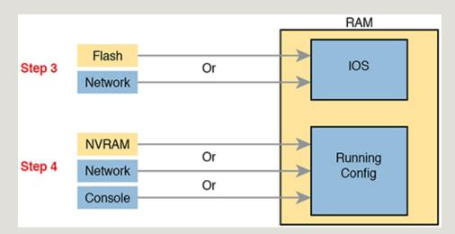
Figure F-3 Loading IOS and Initial Configuration
