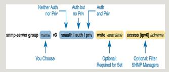
**Figure D-13** SNMPv3 Groups—Configuration Command Parameters
