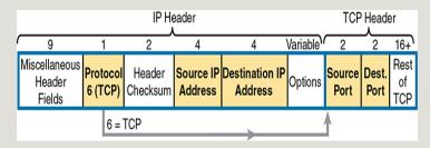
**Figure 11-5** Classification with Five Fields Used by Extended ACLs
