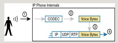
**Figure 11-2** Creating VoIP Packets with an IP Phone and a G.711 Codec
