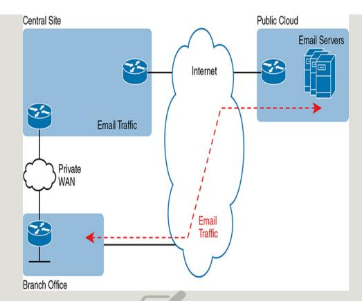
**Figure 15-18** Connecting Branches Directly to the Internet for Public Cloud Traffic
