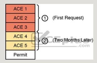
**Figure 17-12** *Lines (ACEs) in an ACL after Two Changes*
