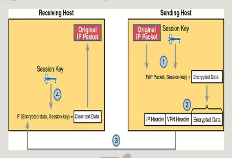
Figure 14-21 Basic IPsec Encryption Process
