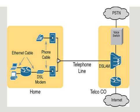
Figure 14-17 Wiring and Devices for a Home DSL Link CEplus
