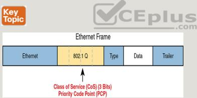
**Figure 11-7** Class of Service Field in 802.1Q/p Header
